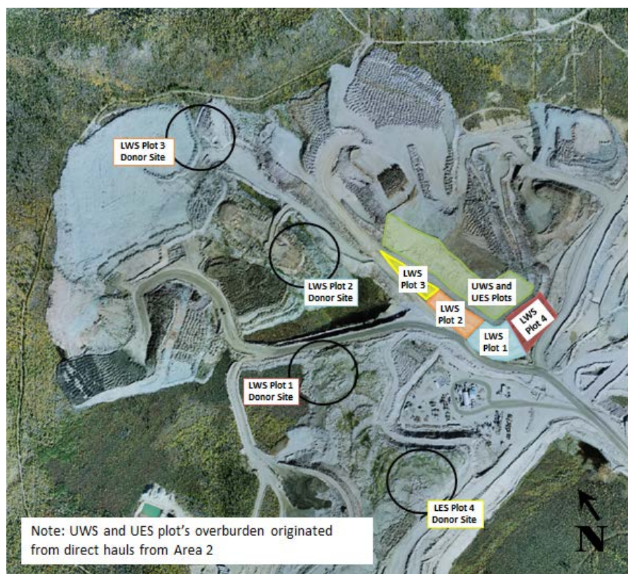
Figure 8-4: Origin of overburden material from Reclamation Overburden Dump placed in distinct plots on the Main Waste Dump re-contoured rock surface.
