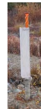
View of SWD-04A; heaved 55 cm out of the ground.
