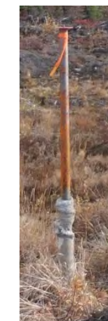
View of SWD-05A; heaved 30 cm out of the ground.
