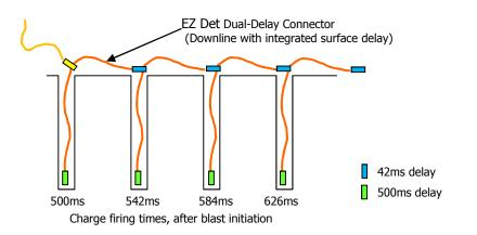
The long in-hole delay element ensures that the much shorter surface delays have time to fire before the ground starts moving: by the time 500ms delays have finished and the powder column is initiated, the surface delay elements are burning several rows further back. This prevents cut-offs, which are incidents in which ground movement tears apart the network of tie-ins before it has had a chance to initiate all of the holes in the pattern.
