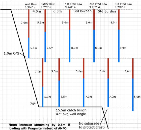
The following table lists hole parameters and the resulting powder factors for each hole type:
