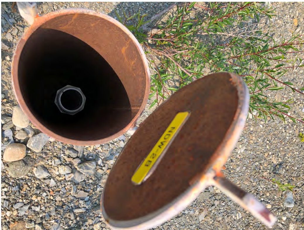
Photo 6: Missing cap on Piezometer NDW-2B
