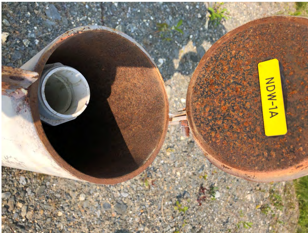
Photo 4: Missing cap on Piezo NDW 1A.
