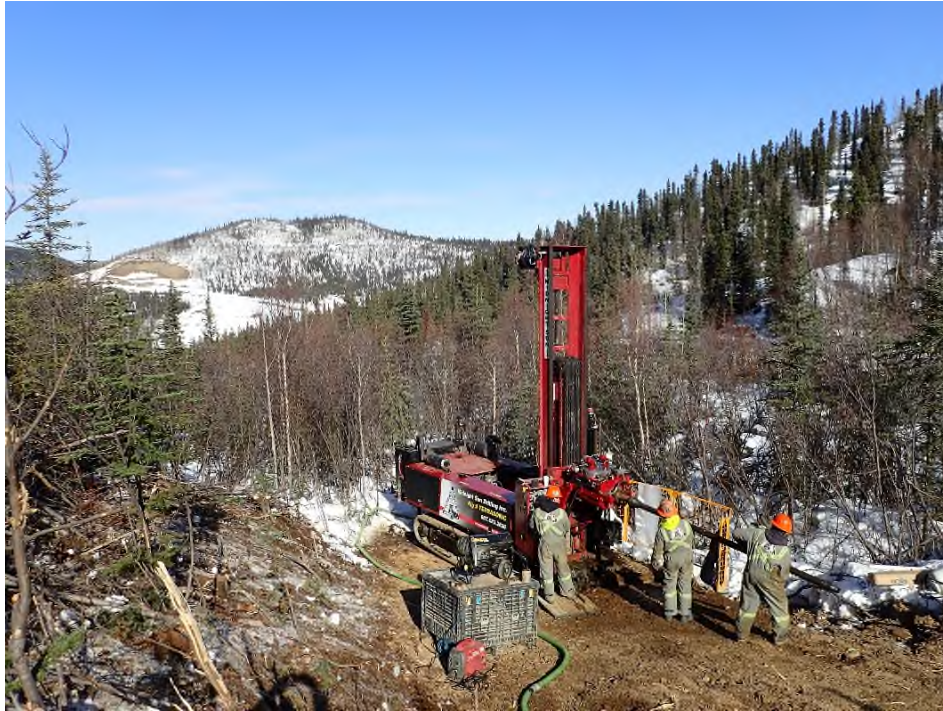
Photo 1: Compact crawler TerraSonic CC150 Drill Rig, Borehole GT18-05 site. Eagle Pup WRSA, looking north. Photo taken April 9, 2018
