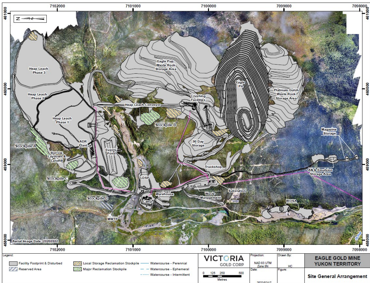
Figure 3-2: Site General Arrangement
