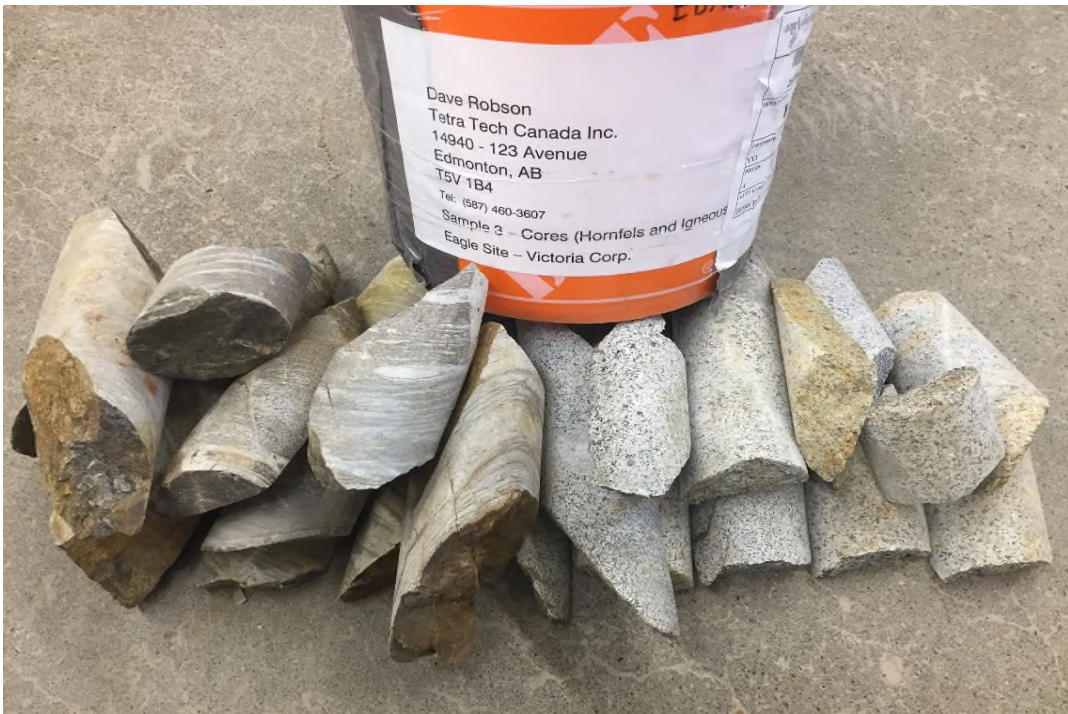
Photo 7: Sample 3 (3a for hornfels and 3b for igneous) that was collected for laboratory durability tests
