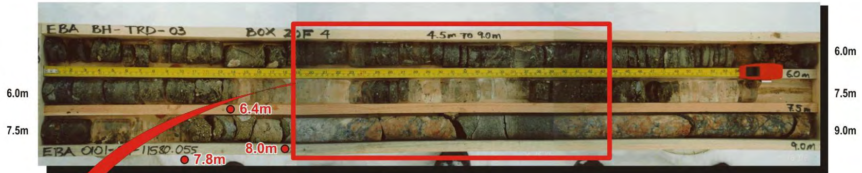
Photo 9: Massive ice bed in perennially frozen till underlain by pegmatite (bedrock). (See Borehole Log: BH 11580-TRD03, Appendix B). ▪ From 4.5 m to 6.4 m: Ice and Gravel and Silt; ▪ From 6.4 m to 7.8 m: Ice ▪ From 7.8 m to 8.0 m: Sand and Gravel ▪ From 8.0 m to 9.0 m: Pegmatite (Bedrock).
