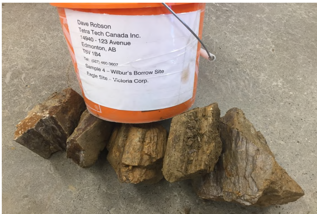
Photo 9: Sample 4 collected for laboratory durability tests
