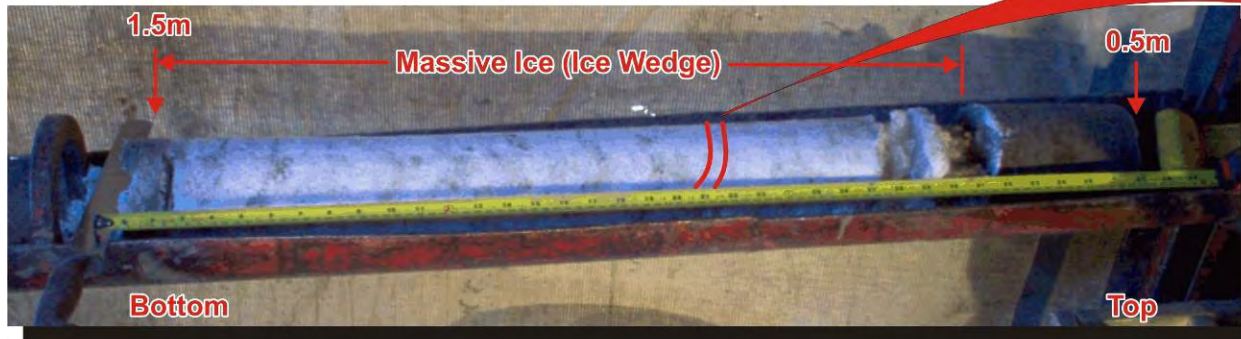
Photo 10a: Core of frozen overburden with ice wedge recovered with a CRREL core barrel. Depth: 0.5 m - 1.5 m.
