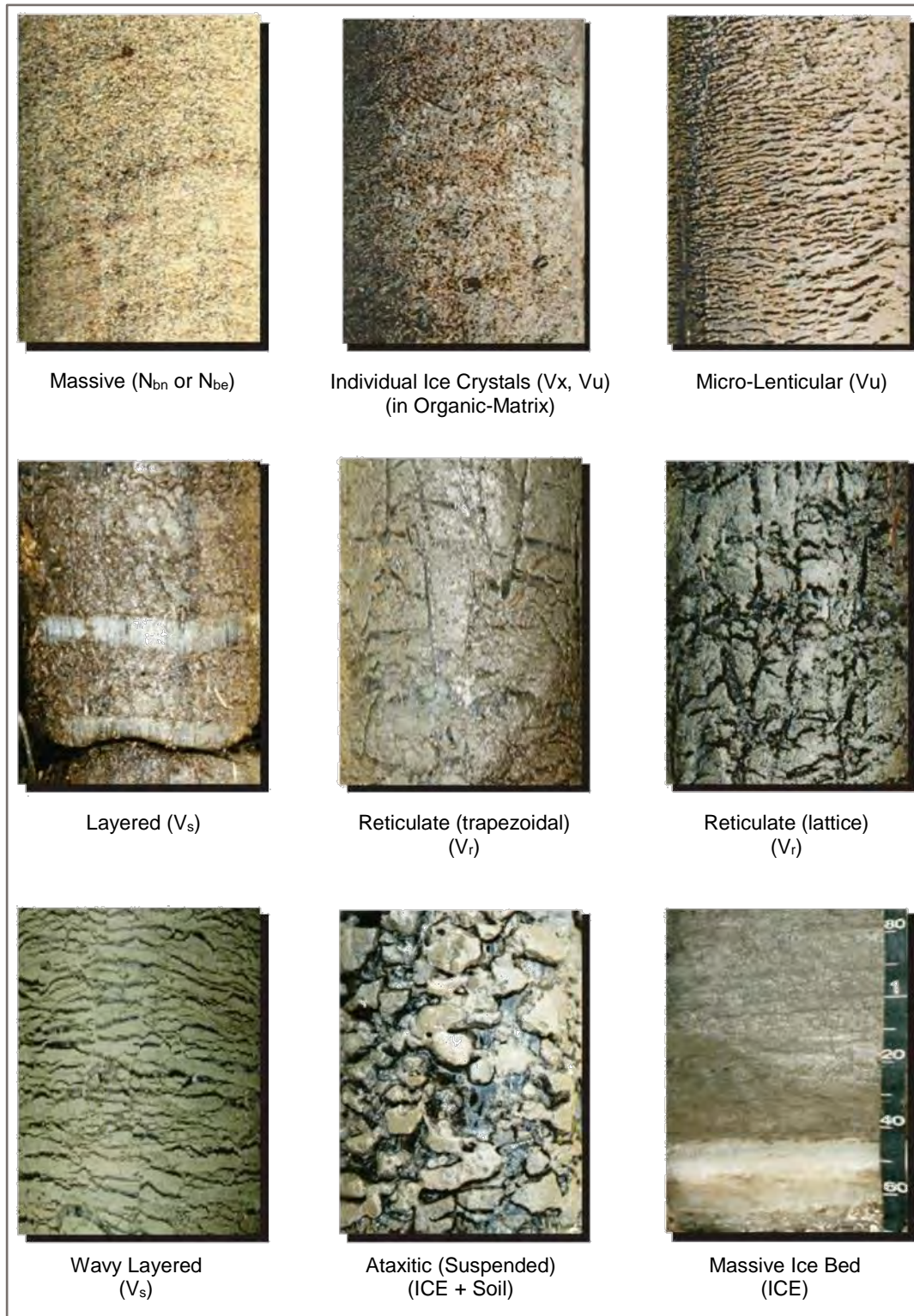
Photo 1: Photographs of simple cryostructures found in perennially frozen soils in the Colville River Delta, Alaska.
