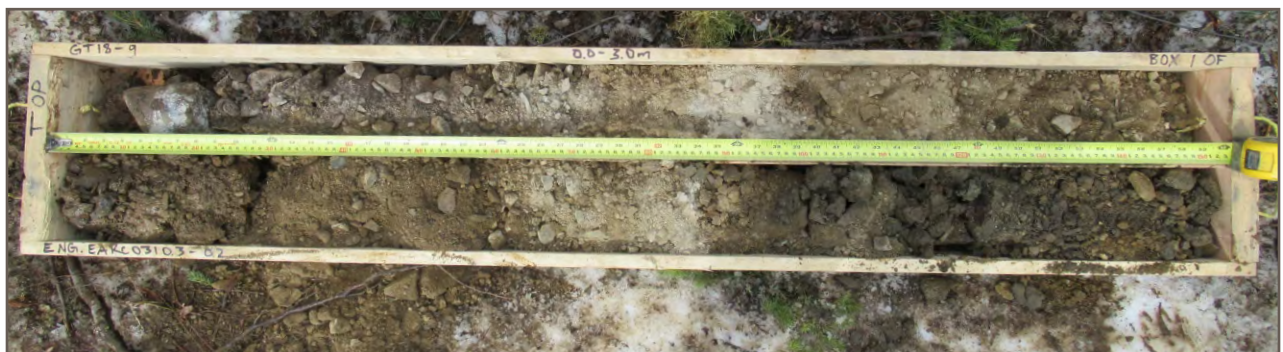
Photo 27: Borehole GT18-09; Depth 0.0 - 3.0 m
