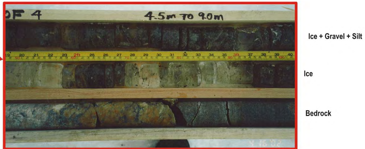
Photo 9: Massive ice bed in perennially frozen till underlain by pegmatite (bedrock). (See Borehole Log: BH 11580-TRD03, Appendix B). ▪ From 4.5 m to 6.4 m: Ice and Gravel and Silt; ▪ From 6.4 m to 7.8 m: Ice ▪ From 7.8 m to 8.0 m: Sand and Gravel ▪ From 8.0 m to 9.0 m: Pegmatite (Bedrock).
