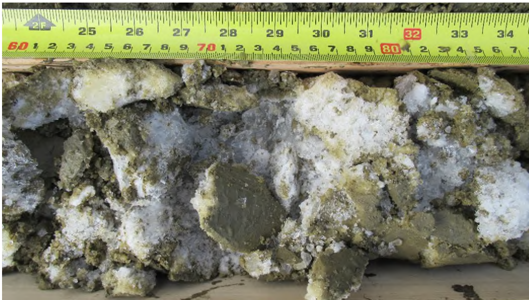
Photo 2: Ice and sand, silty between 1.05 m and 1.2 m in GT18-07.
