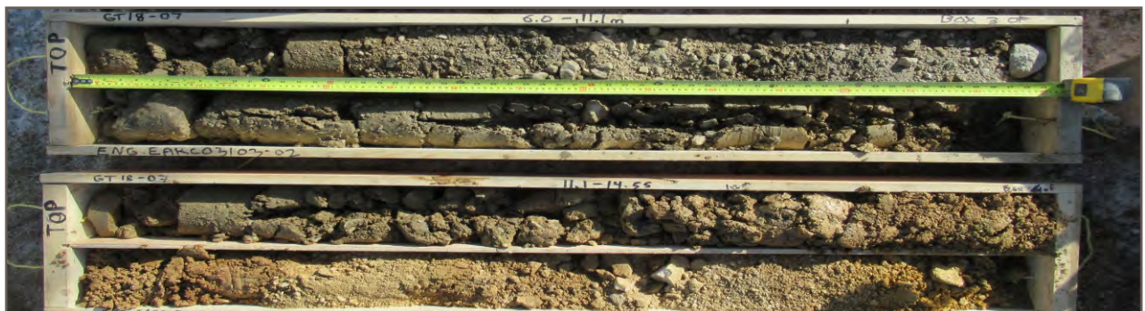
Photo 21: Borehole GT18-07; Depth 6.0 - 14.55 m
