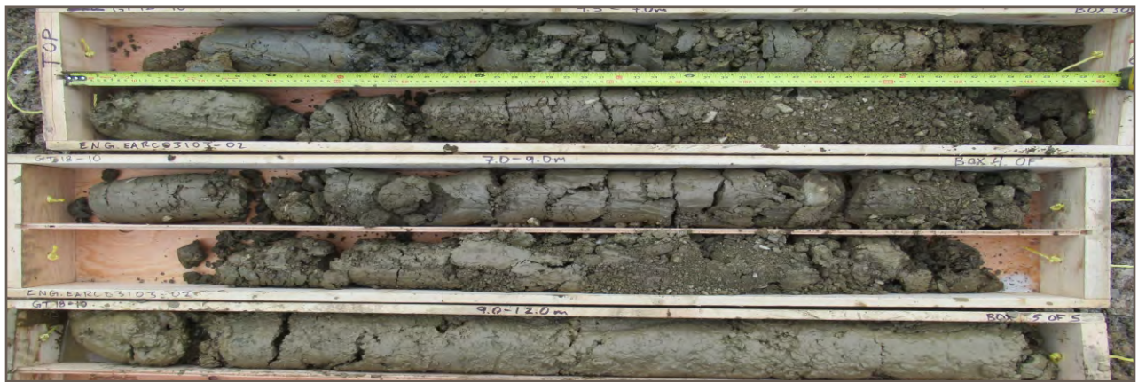
Photo 32: Borehole GT18-10; Depth 4.5 - 12.0 m
