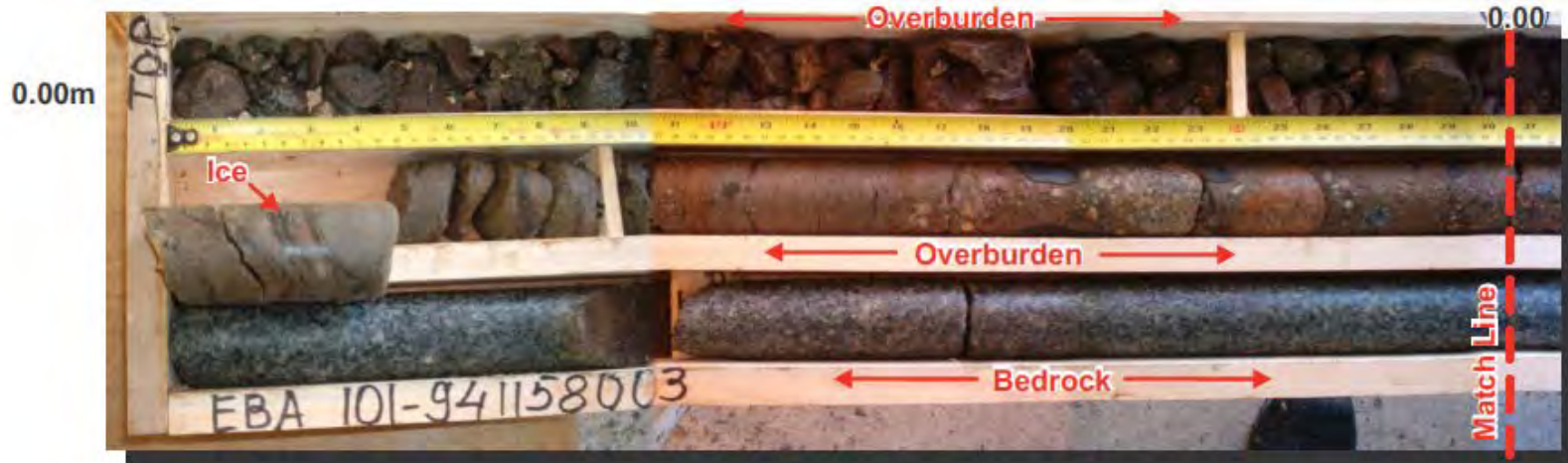
Figure 2a BH 11580.093-03 Core of Frozen Overburden Underlain by Frozen Granite Bedrock (left portion of the core box). Depth: 0.0m - 5.2m
