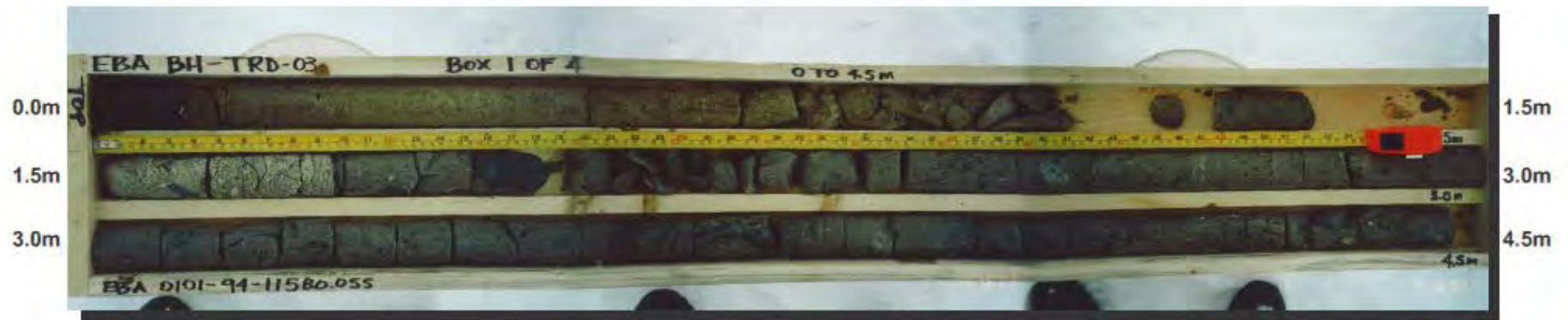
Figure 1a BH 11580-TRD03 Core of Frozen Overburden. Depth: 0.0m - 4.5m.
