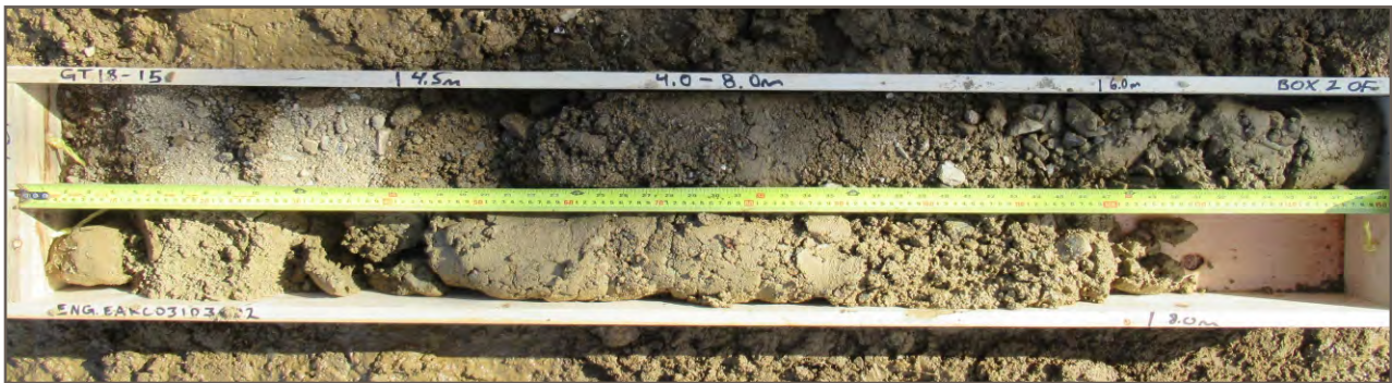
Photo 36: Borehole GT18-15; Depth 4.0 - 8.0 m
