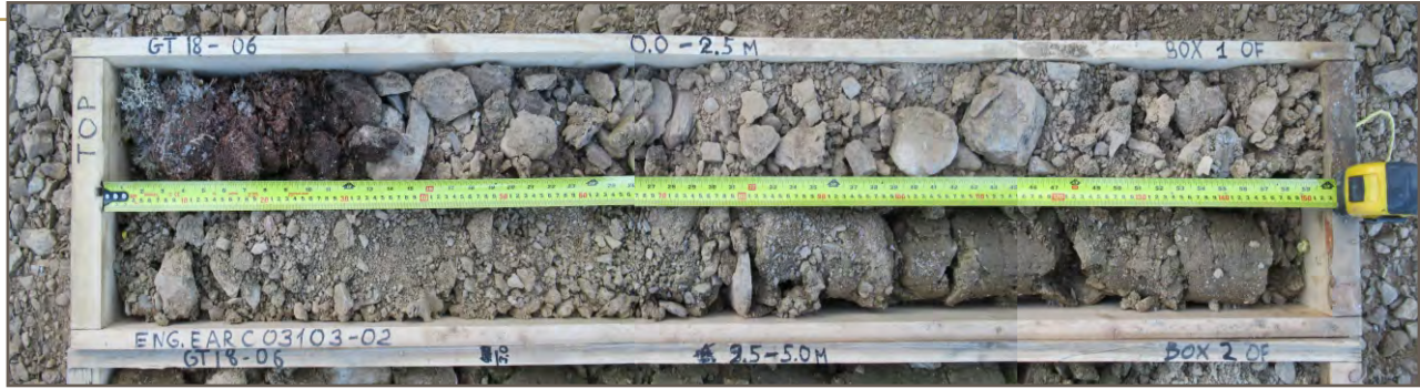
Photo 16: Borehole GT18-06; Depth 0.0 - 2.5 m
