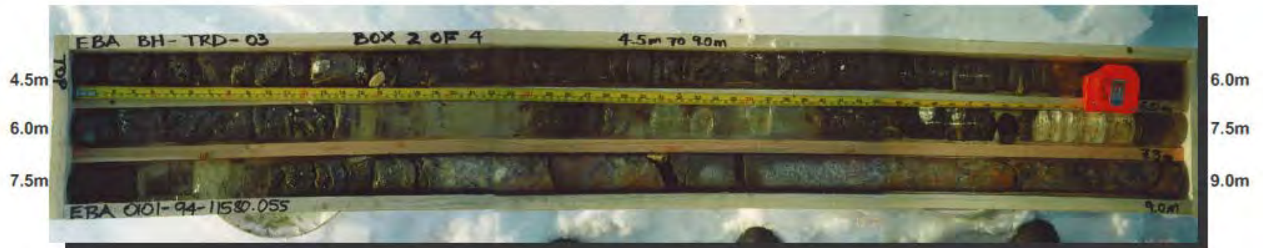
Figure 1b BH 11580-TRD03 Core of Frozen Overburden Underlain by Frozen Bedrock (Pegmatite). Depth: 4.5m - 9.0m.
