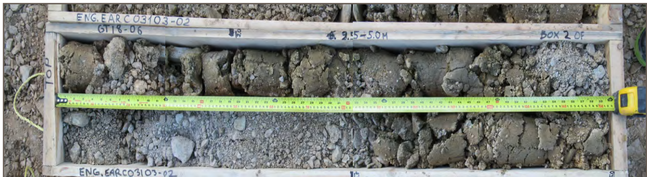
Photo 17: Borehole GT18-06; Depth 2.5 - 5.0 m
