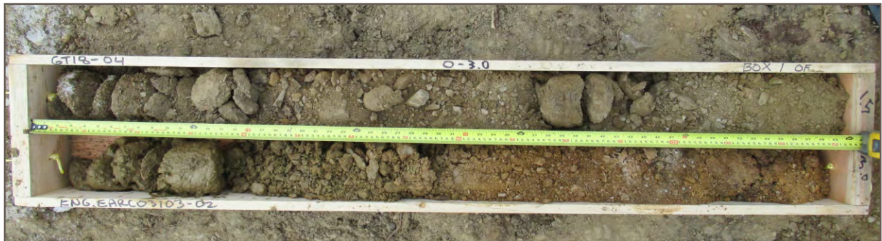
Photo 9: Borehole GT18-04; Depth 0.0 - 3.0 m
