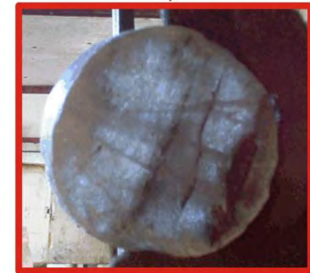
Close Up Slice of an ice core. Note soil (silt) inclusions oriented vertically along vertical cracks in the ice.
