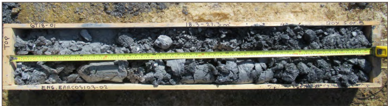
Photo 5: Borehole GT18-01; Depth 18.3 - 21.3 m
