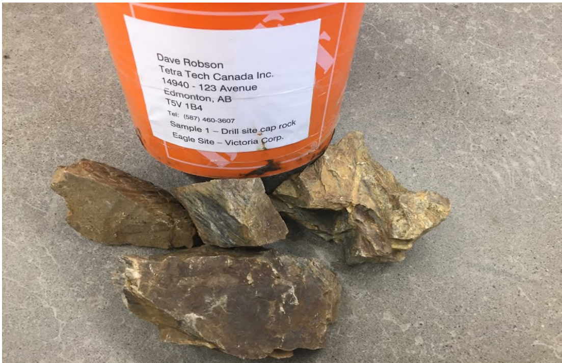
Photo 3: Sample 1 that was collected for laboratory durability tests
