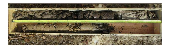
**Photo 23:** Borehole GT18-08; Depth 0.0 - 3.0 m
