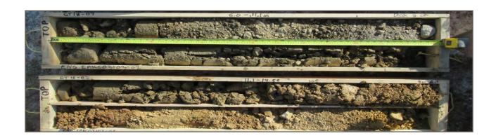
**Photo 21:** Borehole GT18-07; Depth 6.0 - 14.55 m
