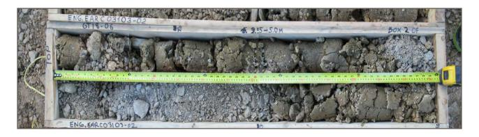
Photo 17: Borehole GT18-06; Depth 2.5 - 5.0 m
