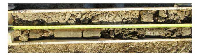
**Photo 12:** Borehole GT18-05; Depth 0.0 - 3.0 m
