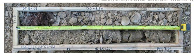
**Photo 16:** Borehole GT18-06; Depth 0.0 - 2.5 m
