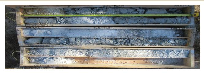
Photo 22: Borehole GT18-07; Depth 14.55 - 21.0 m
