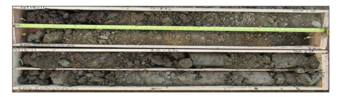
**Photo 33:** Borehole GT18-11; Depth 0.0 - 6.0 m
