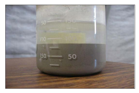
Photo 6: Determining excess ice content in overburden core sample
