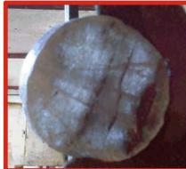
Close Up Slice of an ice core. Note soil (silt) inclusions oriented vertically along vertical cracks in the ice.
