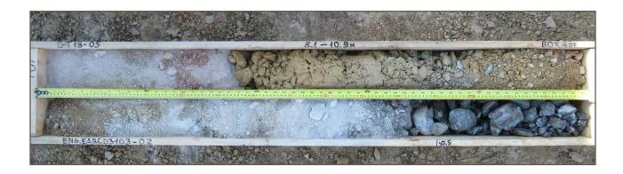
**Photo 14:** Borehole GT18-05; Depth 8.1 - 10.9 m
