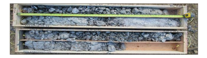
**Photo 15:** Borehole GT18-05; Depth 10.9 - 21.0 m
