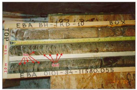
**Photo 3:** Layered cryostructure (Vs 30-40%) in perennially frozen till (at depths of 1.5 m and 3.0 m). Note distinctly oriented ice lenses.
