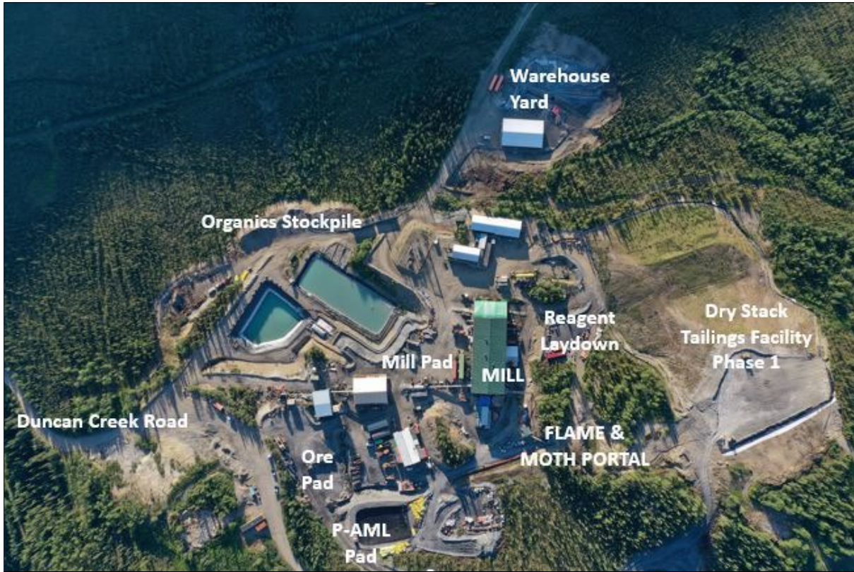
Figure 2-2: Mill and Warehouse Yard Footprint
