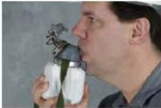
9 Close the lips tightly around the mouthpiece. A tight seal must be maintained throughout escape to safety.
