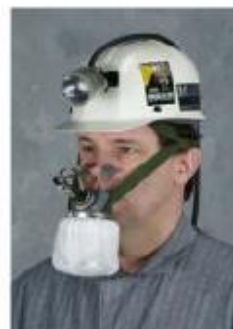
13 Replace headgear. Be sure not to dislodge the head harness. The W 65 Self-Rescuer is now ready for use. Breathing through the device is obviously somewhat more difficult than breathing under normal conditions. This will become more apparent under extreme exertion. Therefore, when escaping, keep calm and avoid exerting yourself too much. If possible, rest for short periods. Be sure you understand the important instructions on page 8.
