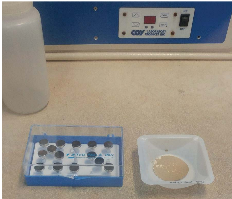
Figure 1. Filter paper and Scanning electron microscopy stubs loaded in an anaerobic chamber
