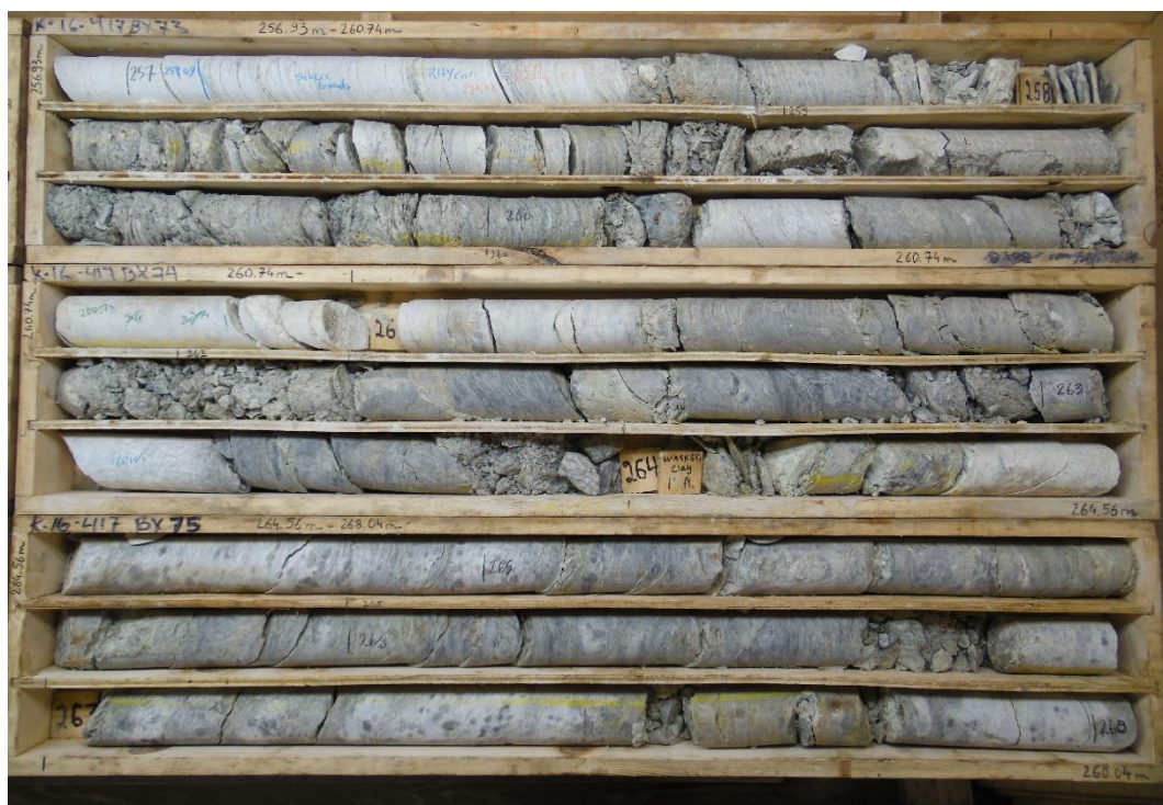
Figure 17 Core photo example of E-W strike geotechnical structure in K17-307
