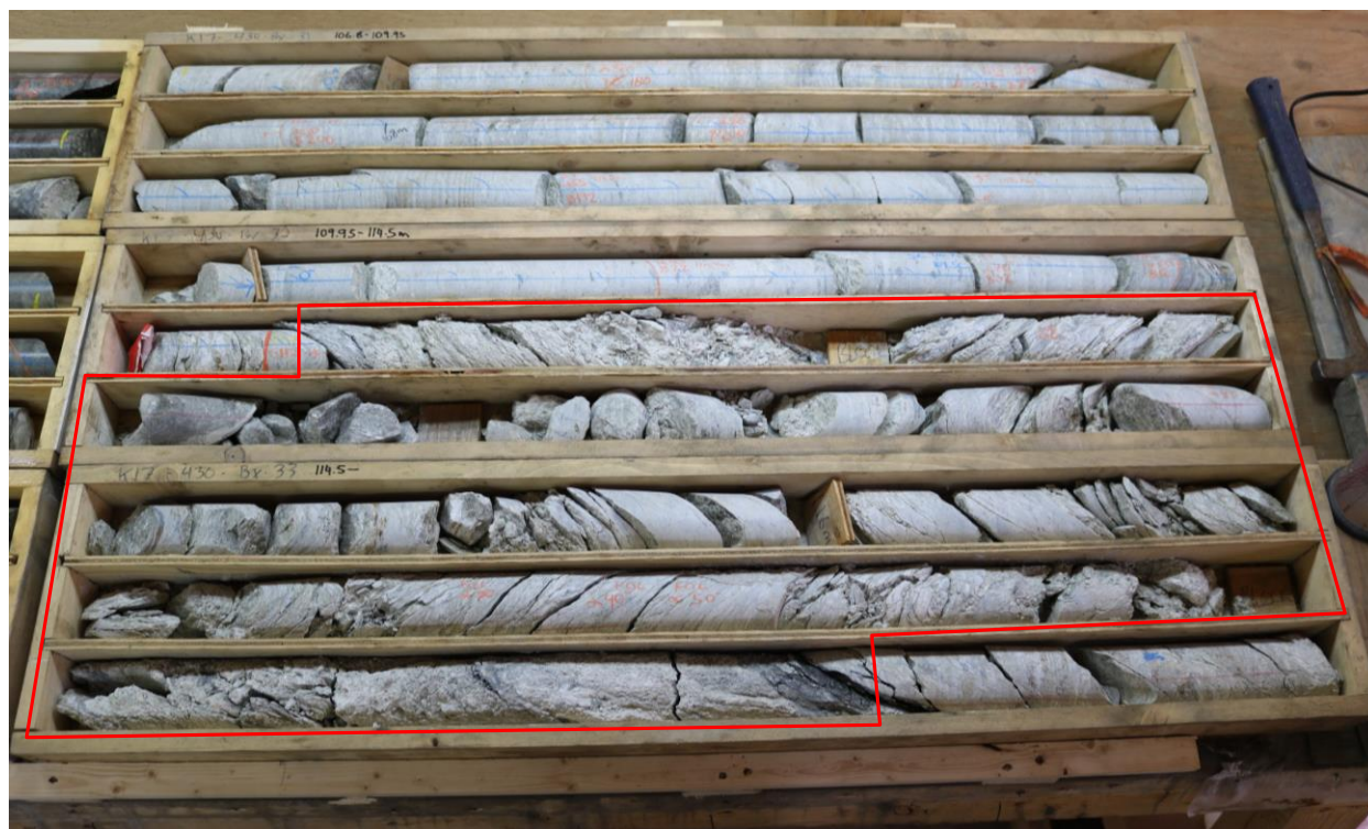
Figure 7 Example of fault zone identified with orientation in televiwer data and core photo in drillhole K17-430
