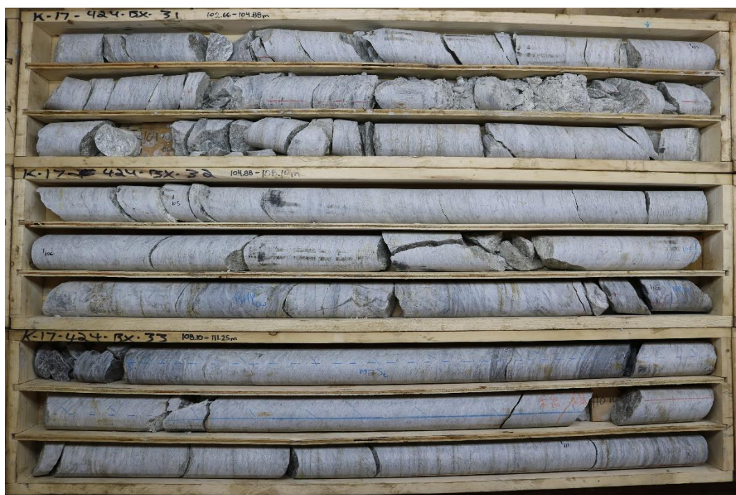
Figure 19 Core photo example of NNW strike geotechnical structure in K17-424
