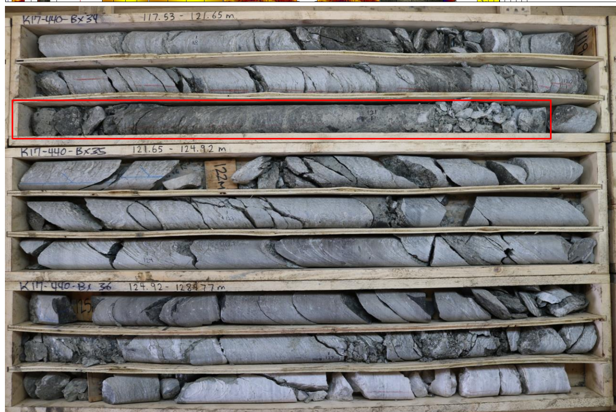
Figure 8 Example of fault zone identified with orientation in televiwer data and core photo in drillhole K17-440
