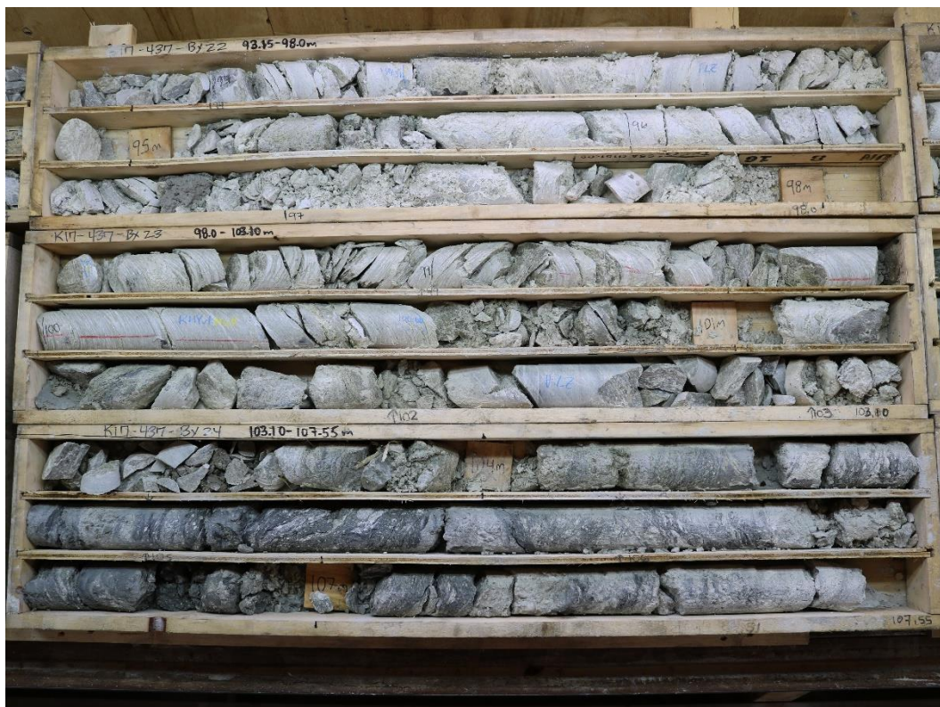
Figure 22 Core photo showing example part of the Creek Fault in K17-424
