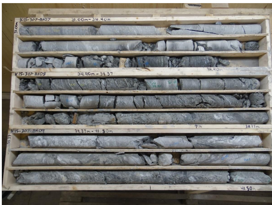
Figure 13 Core photo example of NE strike geotechnical structure in K15-307
