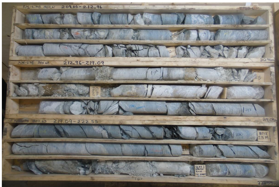
Figure 15 Core photo example of NNE strike geotechnical structure in K15-238
