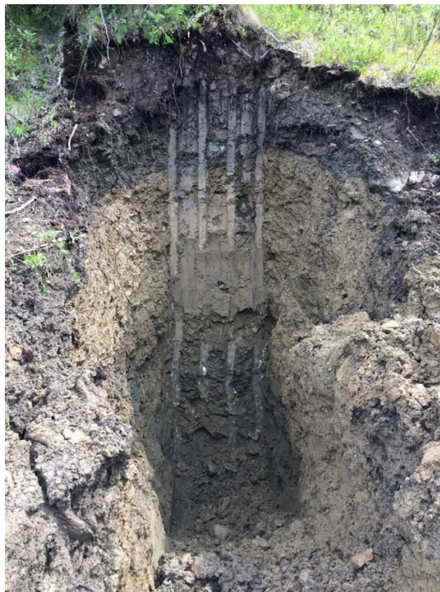
Figure 56: Typical Overburden Profile
