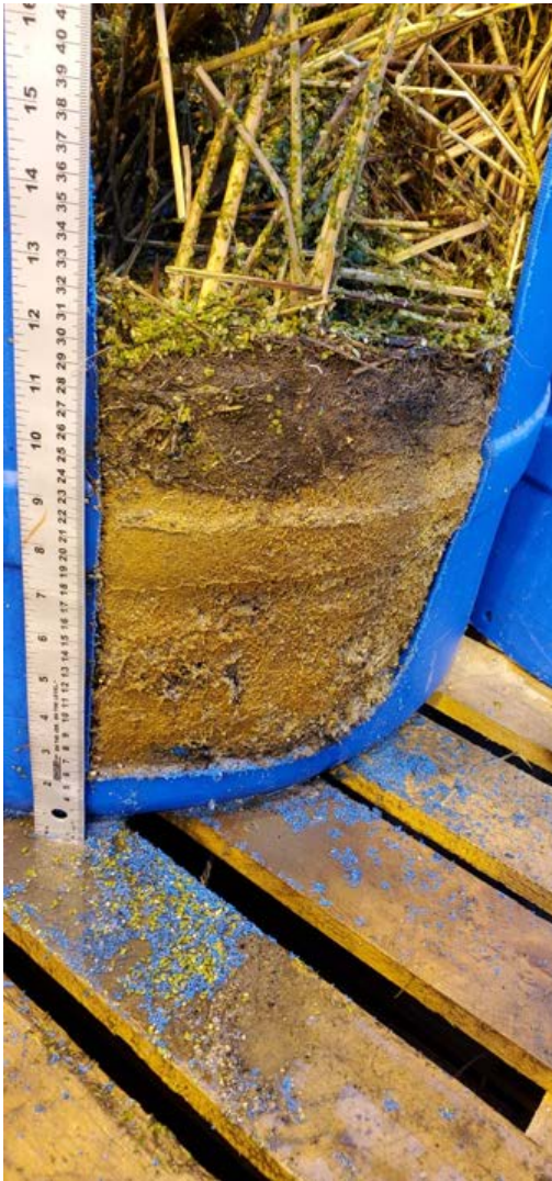
Photograph 8-6: Water Sedge (Left) and Bulrush (Right) Cut Open at the end of Operations Phase to Show Accretion and Root Mats
