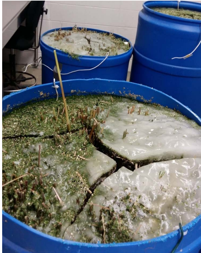
Photograph 6-1: Frozen Constructed Wetland Treatment System Cells Brought Inside for Thawing
