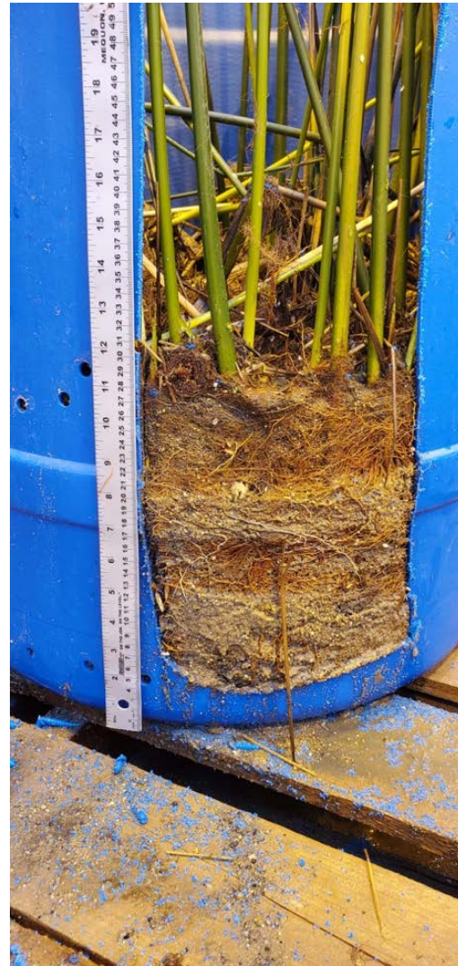
Photograph 8-6: Water Sedge (Left) and Bulrush (Right) Cut Open at the end of Operations Phase to Show Accretion and Root Mats
