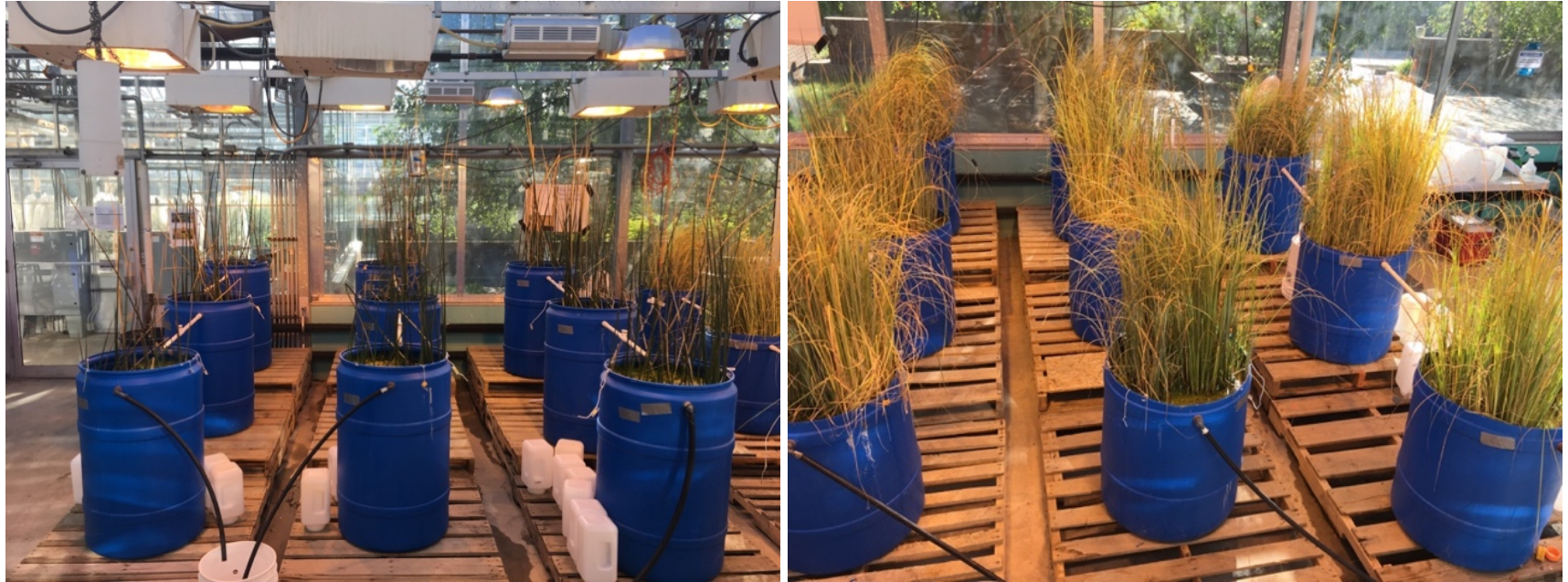
Photograph 8-3: Off Site Pilot-scale Constructed Wetland Treatment Systems on August 23, 2019
