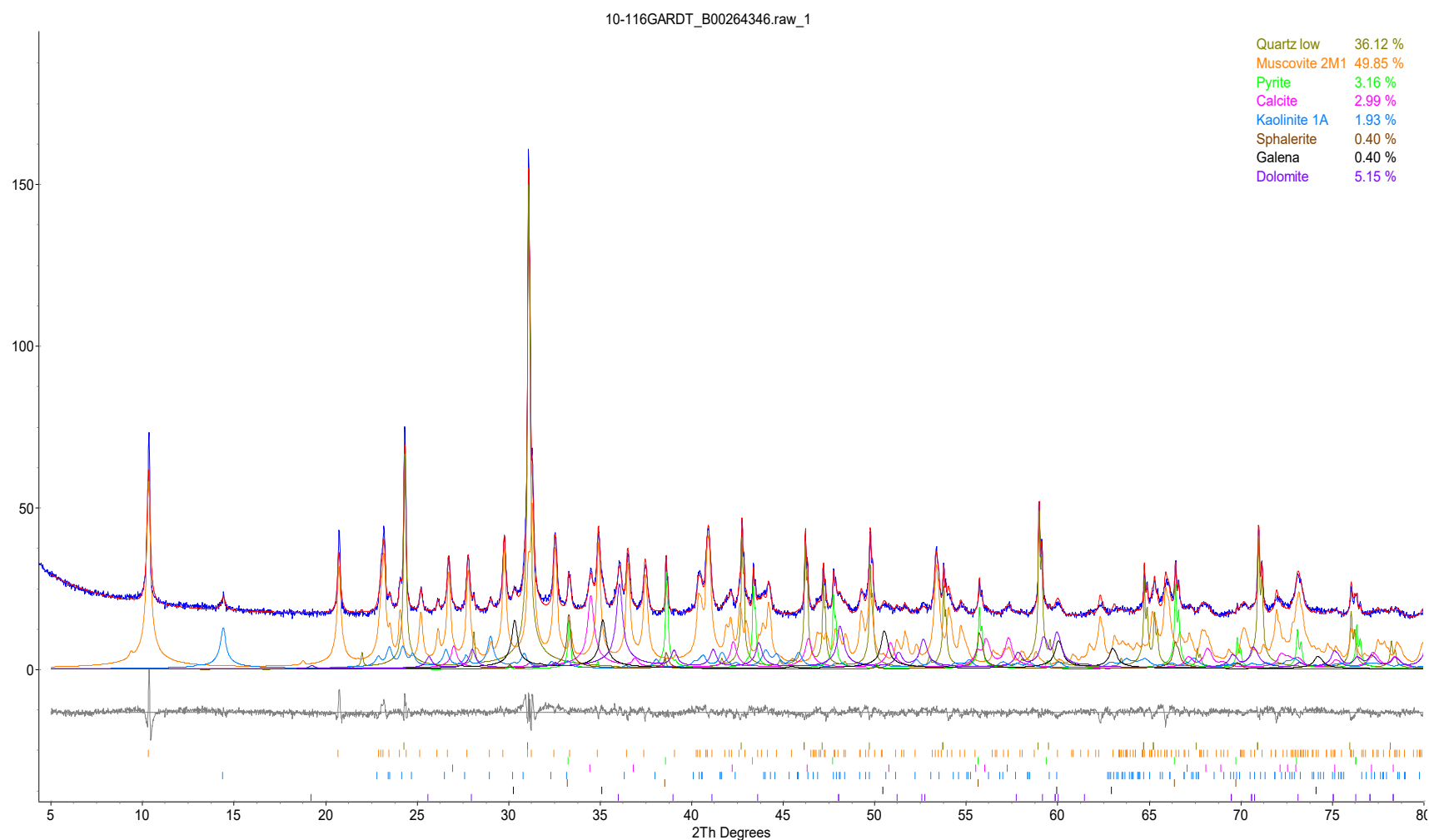
Figure 10. Rietveld refinement plot of sample Global ARD Testing Services 116: B00264346 (blue line - observed intensity at each step; red line - calculated pattern; solid grey line below – difference between observed and calculated intensities; vertical bars, positions of all Bragg reflections). Coloured lines are individual diffraction patterns of all phases.
