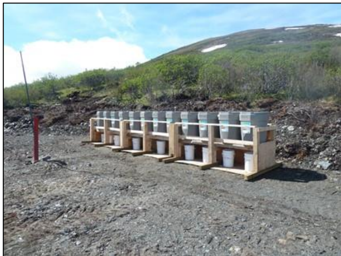
Figure 4-6: Field Leach Barrel Setup
