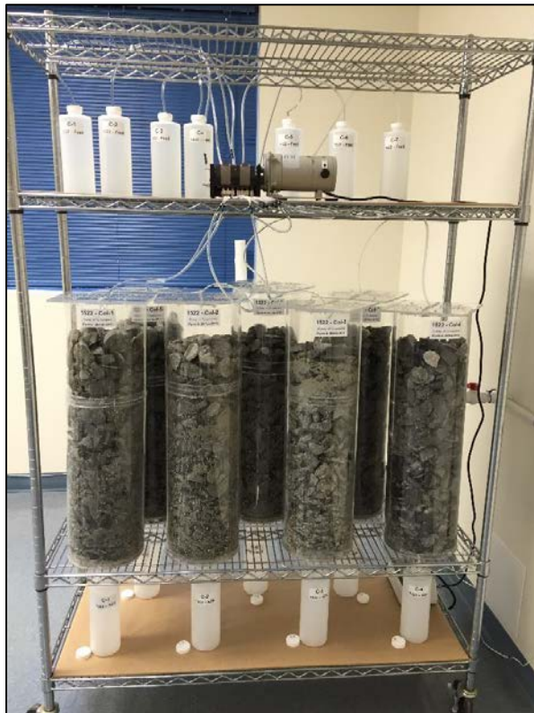
Figure 4-5: Trickle Leach Columns (left) and Humidity Cells (right) Setup
