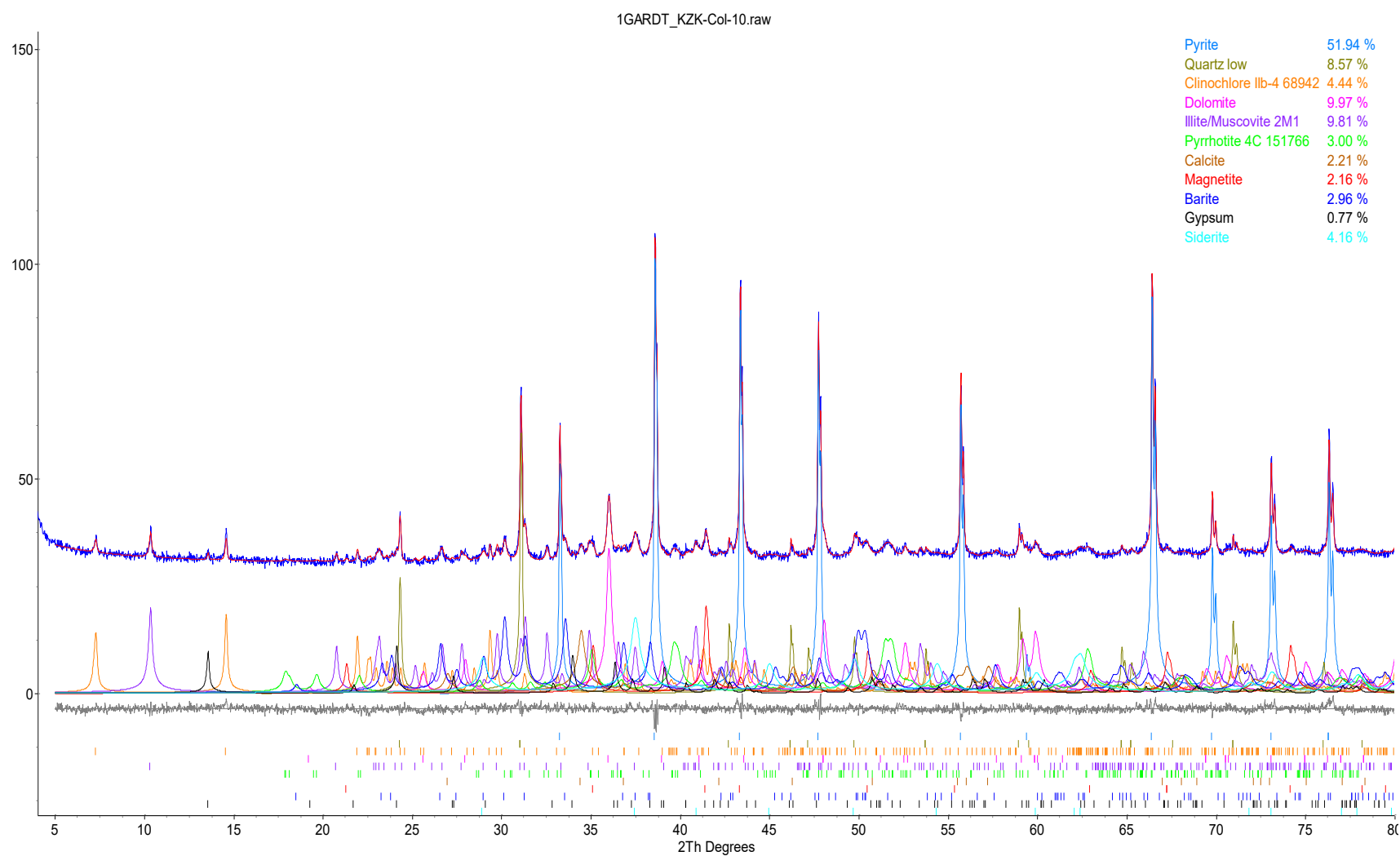
Figure 1. Rietveld refinement plot of sample Global ARD Testing Services KZK- A17107 (Test #1-20) (blue line - observed intensity at each step; red line - calculated pattern; solid grey line below – difference between observed and calculated intensities; vertical bars, positions of all Bragg reflections). Coloured lines are individual diffraction patterns of all phases.
