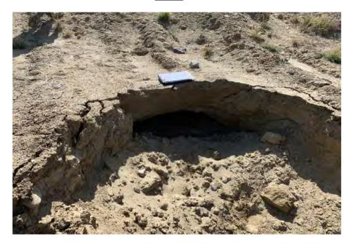
Photo 1: Ponded water drained through "rathole"
