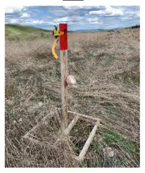
Photo 3: Extensometer that remains, No movement since 2017.
