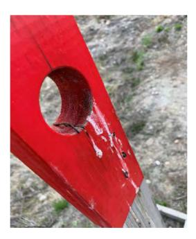
Photo 4: Western extensometer, wire has broken, but no apparent movement.
