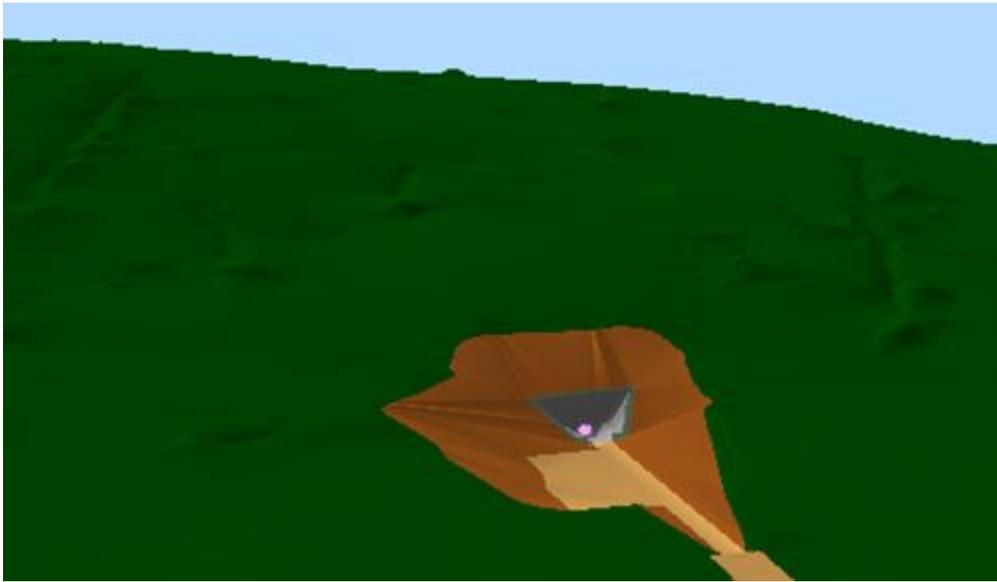
The rock trench will be supported as required and will at a minimum have 2.4 metre long #6 resin grouted rebar installed on a 1 metre by 1 metre spacing with welded wire mesh on the portal face.
