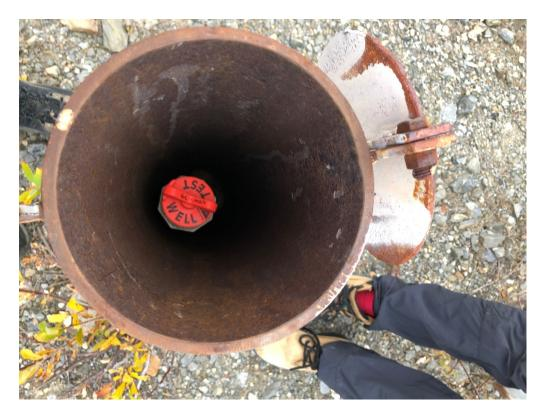
Photo 3: Typical North Dam Piezometer
