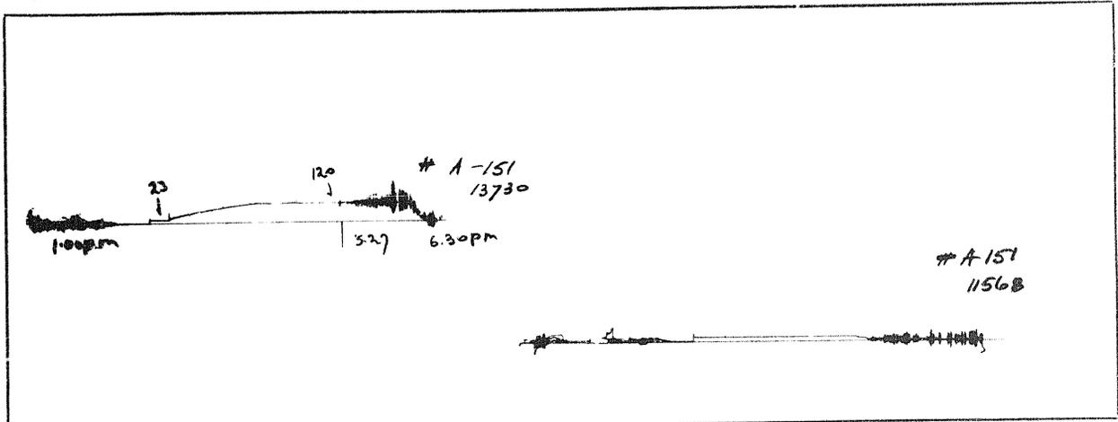
RECORDER No 13730... ELEMENT RANGE 0-2200... P.S.I. CLOCK SPEED: 12 HRS. RECORDER DEPTH 2684'
